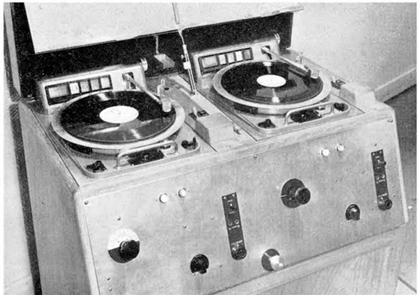
A BBC-designed record player. Like its predecessors it has a "drop-start" and prefade on headphones, so that records can be set up without fading up. It has windows for the optical groove locating unit and speed selection indicators. If the wrong stylus is chosen they all light up together and flash! Unlike earlier record players, the stylus of the RP/2 cannot easily be seen; a slight disadvantage when time is pressing. But the quality from the moving coil pick-up is excellent
