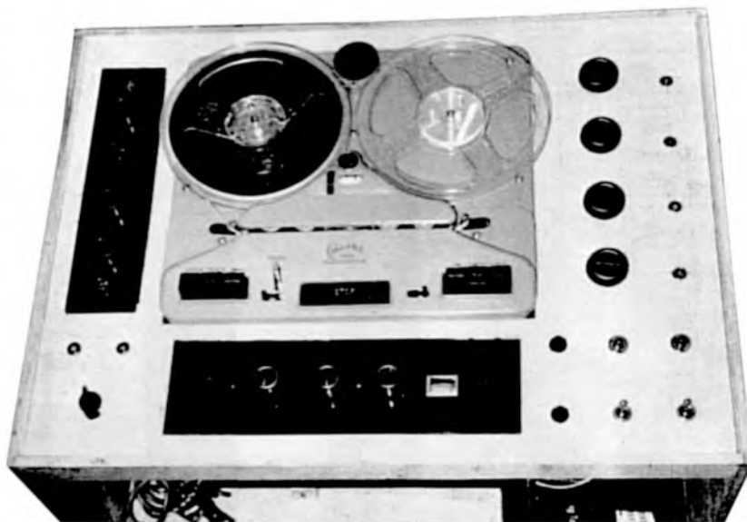
The home-built tape recorder described in this article
